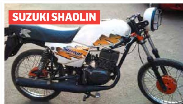
SUZUKI SHAOLIN My old 1988 Suzuki Shaolin, at 12bhp it had the first five-speed gearbox on a bike sold in India. Meskin Moses
