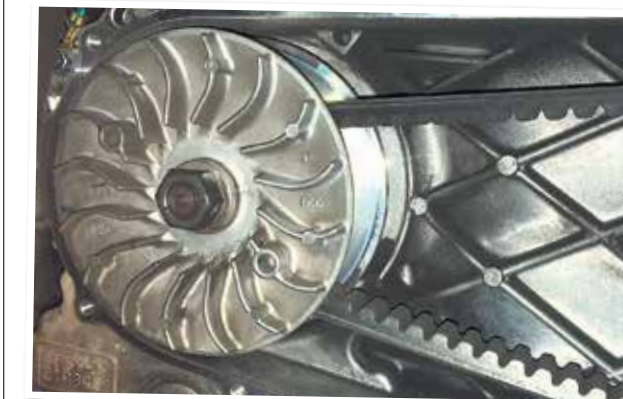
Toothed belt is the equivalent of a final drive chain on most bikes
