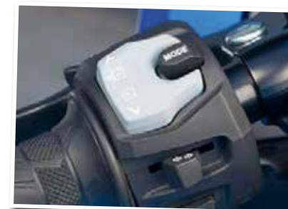
Improved position of mode button prevents unintentional switching
