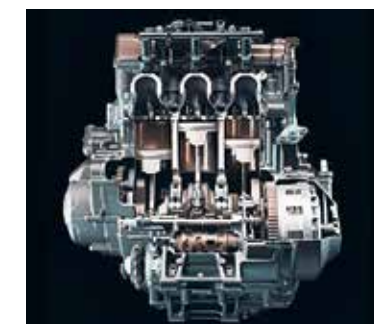
Triples never have more than two pistons sitting at top dead centre
