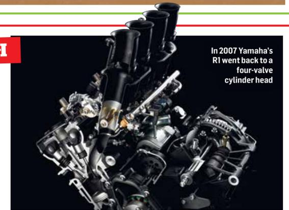
In 2007 Yamaha's R1 went back to a four-valve cylinder head
