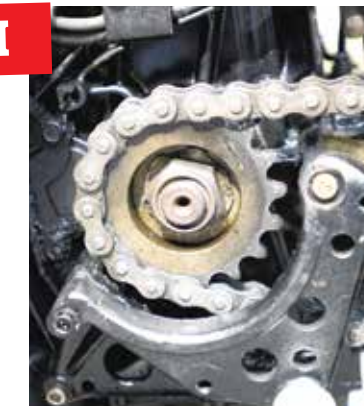
Go too small with the front sprocket and you'll feel pulsing in the chain
