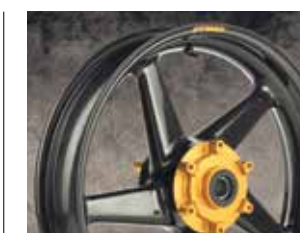
Dymag's carbon fibre wheels have an aluminium hub
