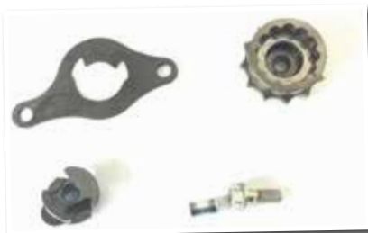
The pin that links the gear change to the shift drum on an NC750 can wear, sticking the bike in gear
